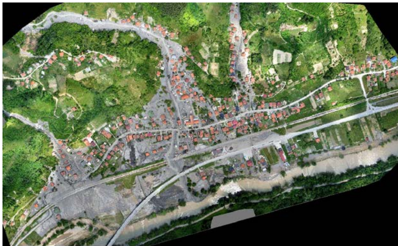
Figure 15 - Montage of aerial imagery and a 3D photogrammetric model of the debris flow at Topčić Polje (Peter Spruyt, European Commission Joint Research Centre - JRC)
