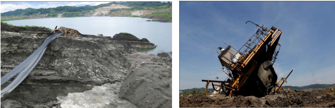
Figure 3 - Damaged heavy equipment and flooded open cast mine at 'Sikulje', Kreka
